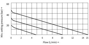
$P_{Amin}$ -Q Characteristic curve shows the flow-rate in relation to the adjustable min. pressure rating from P to A.
